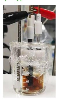
An electrochemical setup to transform lignin
